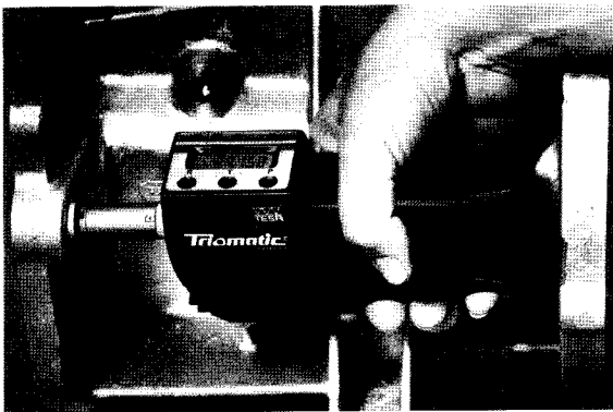
FIGURE 35.12 An electronic gage for measuring bore diameters. The measuring head is equipped with three carbide-tipped steel pins for wear resistance. The LED display reads 29.158 mm. Source: Courtesy of TESA SA.
